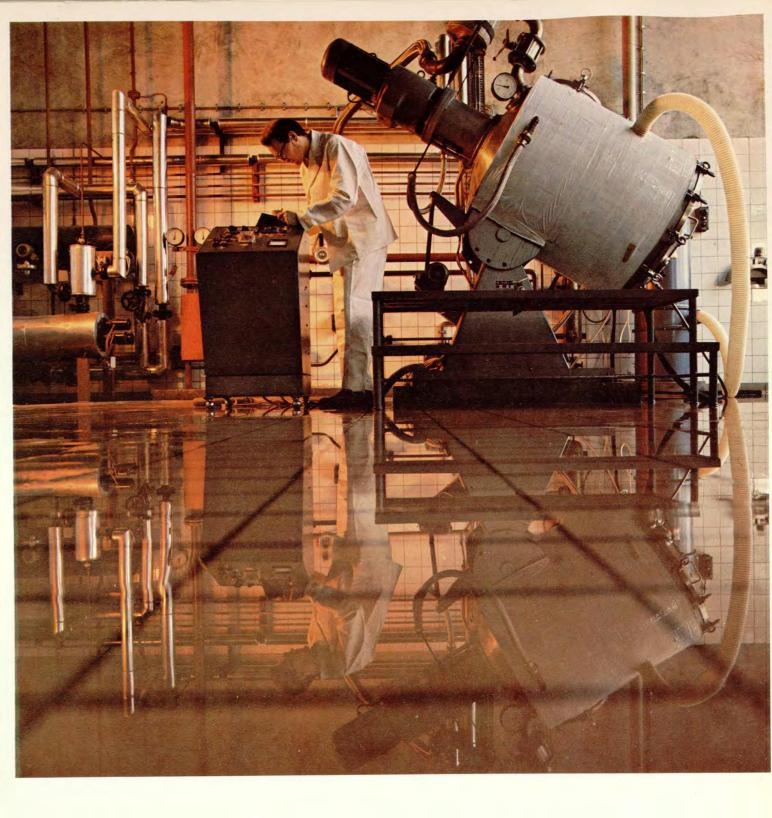
n.v. Organon has acquired a topo granulator for pretreatment of pharmaceutical substances to be included in tablets. This newly developed apparatus greatly simplifies the production process.
