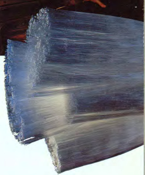
In an industrial dialysis process, Akzo membranes remove alcohol from beer while leaving the taste in.
