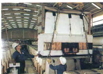
Asbestos diaphragms in the Delfzijl, the Netherlands, electrolysis plant are being replaced on trial by plastic diaphragms.
