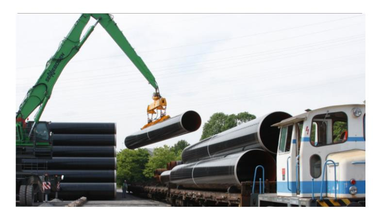
AkzoNobel provided powder coatings for the 1,223-kilometer long Nord Stream gas pipeline. Due to be operational in 2012, the pipes have been coated with a Resicoat primer for a three-layer system. In total, 1,500 tons of coatings were delivered for the project.
