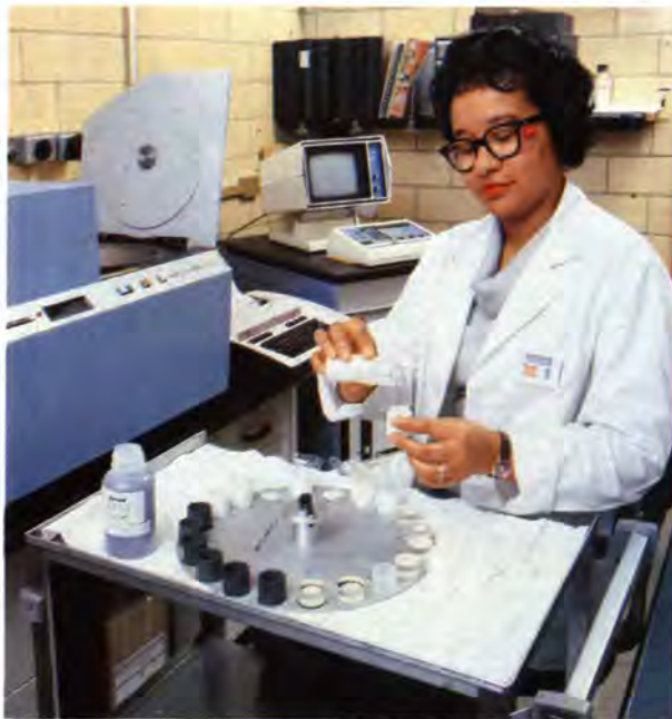
Research technician of American Enka (Aktiona) prepares samples for analysis by means of an X-ray fluorescence spectrometer.
