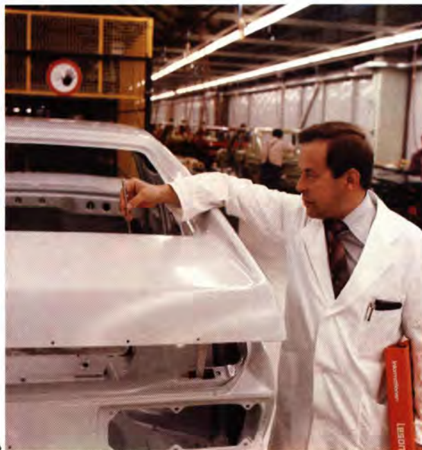
Inspector of Deutsche Akzo Coatings measures thickness of paint coat on auto body in automobile manufacturing plant.
