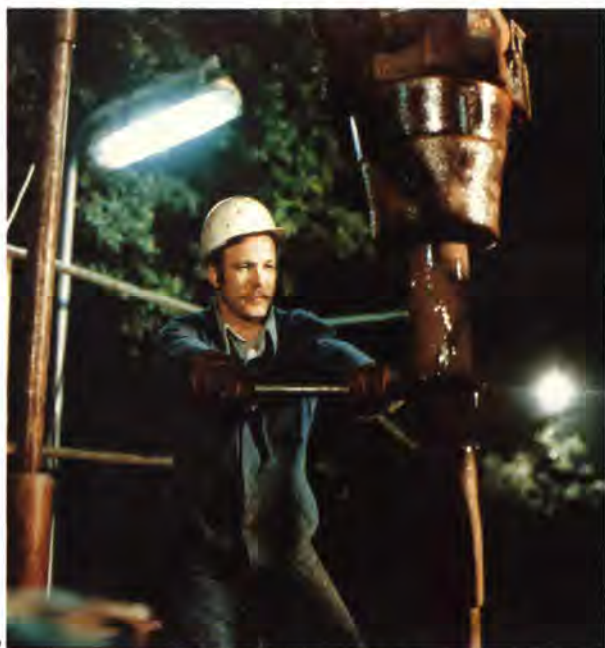
» Drilling operator of Akzo Zout Chemie in Hengelo (the Netherlands) sinks well into salt bed through which salt will be brought to the surface in solution.
