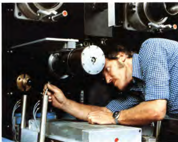
» Technician of Barmag Barmer Maschinenfabrik (West Germany) works on assembly of integrated spin-draw-texturing machine for carpet yarns.
