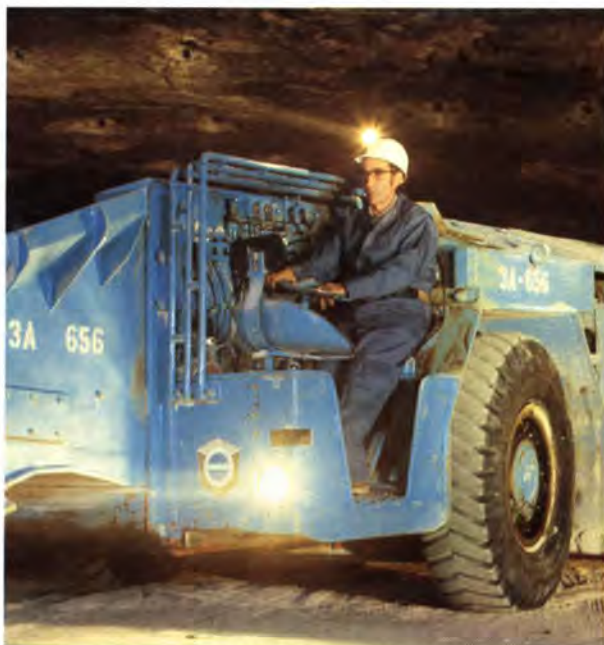
Operator in International Salt (Akzona) mine drives 20-ton capacity diesel-engined shuttle car carrying rock salt from the faces to the crushers.
