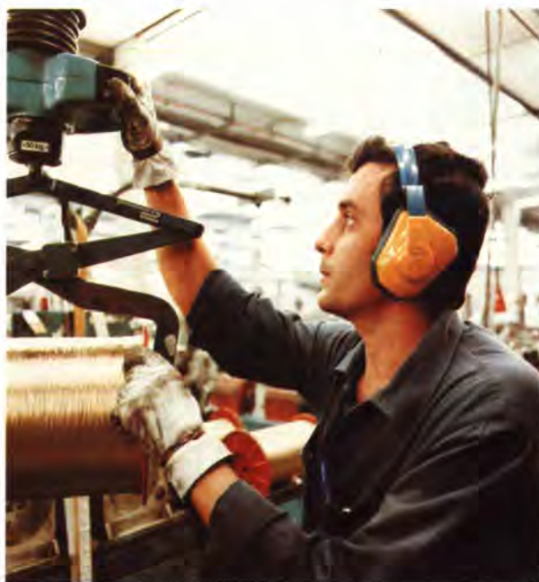
» Patrol man in the Enka steel cord plant at Oberbruch (West Germany) uses lifting device in doffing completed spools weighing some 40 kg each.
