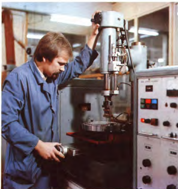
» Technician of Enka tecnica, of Oberbruch (West Germany), machines orifices in spinneret of the type used in the production of polyester staple in Enka plants.
