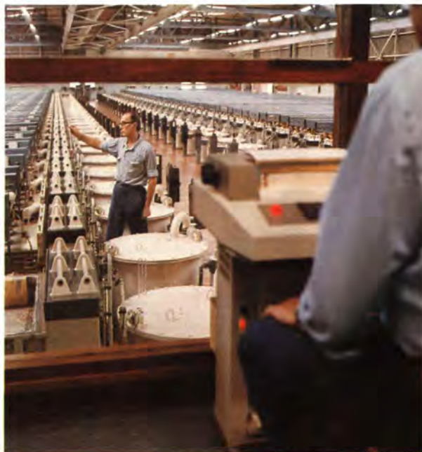
» Process operator tests quality of caustic soda in the cell room of Akzo Zout Chemie's electrolysis plant at Hengelo (the Netherlands).
