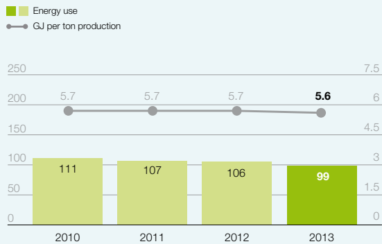
Energy use [TJ] is the sum of fuels, electricity, steam, hot water and other utilities (expressed as fuel equivalents).
